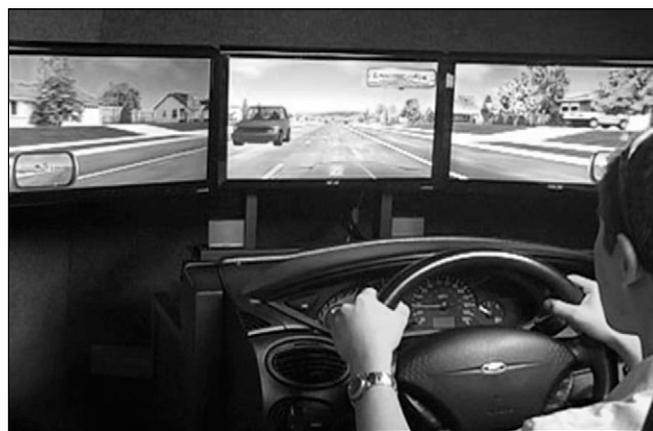
**Figure 1.** The DriveSafety DS-250r<sup>™</sup> Driving Simulator with three 20-in. panels for a 65° field of view, engineered into the cargo area of a 2010 Dodge Caravan.
