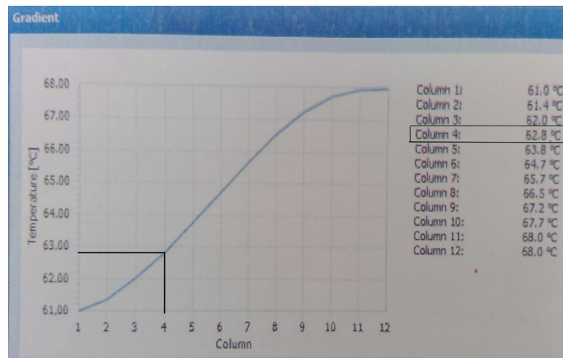
Figure 3: Temperature Gradient Analysis performed on the LC96. Same samples: 1 Positive and 1 Negative Control run repeatedly from column 1 to 11 with temperature range set at 61°C –68°C. Non-Template Control run at column 12). Column 4 at 62.8°C is where highest \Delta Ct value was detected.
