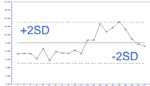
Figure 5: Plot of \Delta C_t precision data. X-axis = Sample Replicates, Y-axis = \Delta C_t values (from Table-9). Horizontal central line indicates the mean of the \Delta C_t values.
